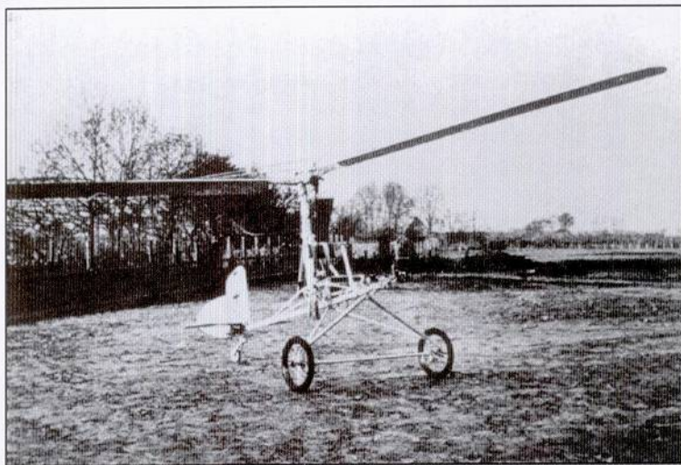
Prototype gyroglider Fa 330 Bachstelze on wheeled undercarriage.
