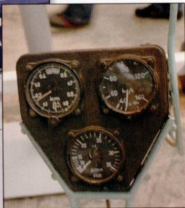
Above: Instrument panel of the Fa 330.
