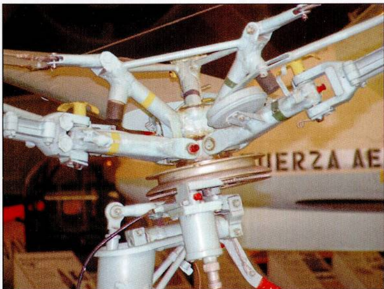
Details of the Fa 330 rotor head.
