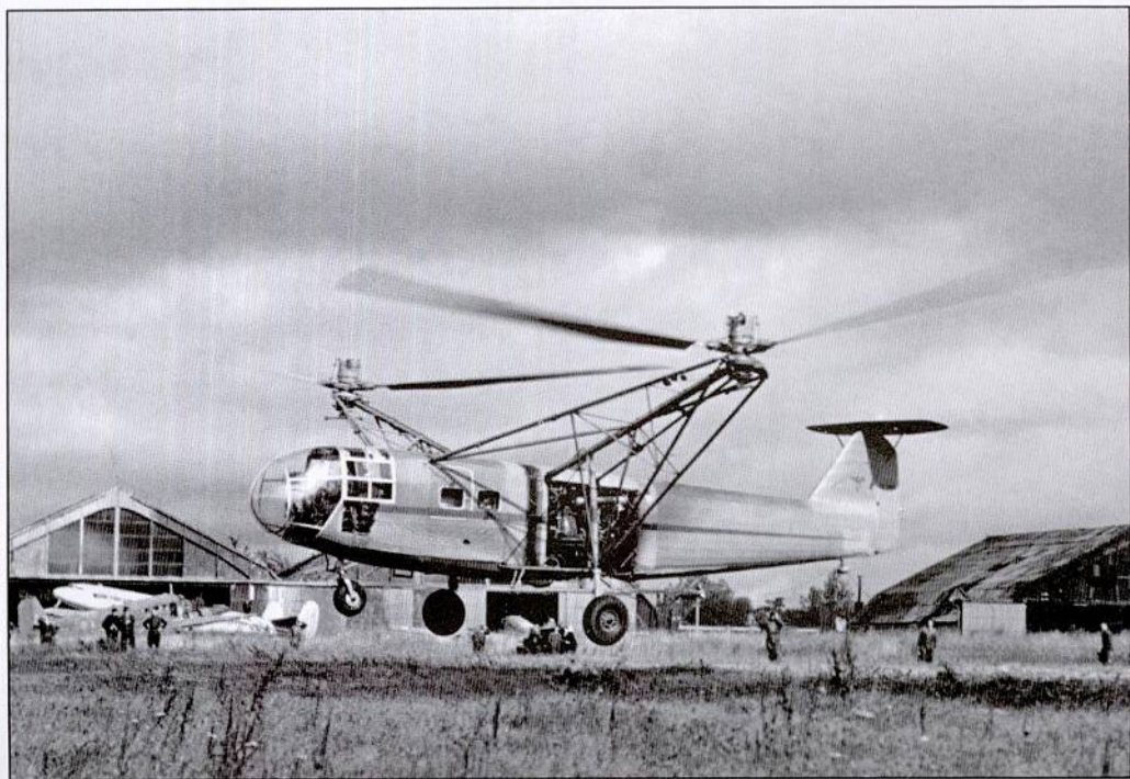
SE 3000, the French version of the Fa 223, Drache during factory tests (1948)
