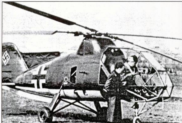
The third prototype F1 282, V3 GF+YC. Cockpit glazed at the front only.
