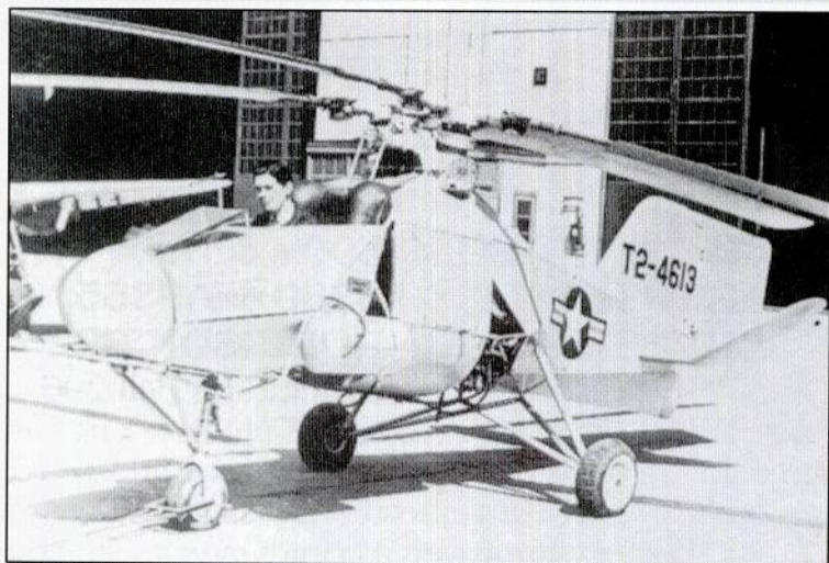
Fl 282B-2 Kolibri V23 during evaluation in the USA, with American markings. [HelicoRevue]
