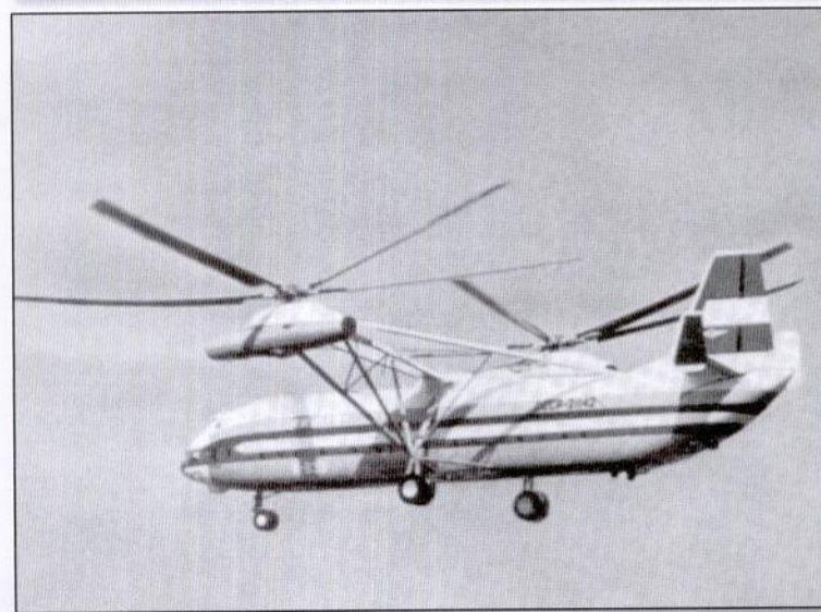
The Soviet Mi-12 of 1967, the biggest helicopter in the world, built in the lay- out of the historical Fw 61. [R. Witkowski Archive]
